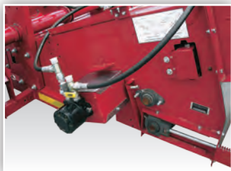
Hydraulic Drive (shown with optional valve kit)
